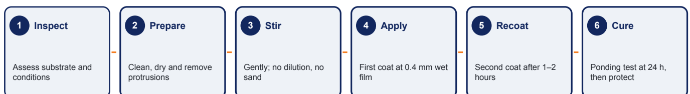
Figure 2 — Application workflow. Each stage is a hold point: confirm the previous stage is complete and within specification before proceeding.
